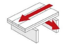
• Check with the joist or truss Manufacturer to determine if cross-bracing is allowed with that system. Should it not be compatible with the joist or truss Manufacturer, sheeting the sub floor with a second layer of CD or better grade plywood would then be the only option. (See double layer sub floors section).
