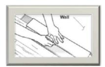
Cut a piece that is a least 5.9" or 150mm shorter than the first plank to start the second row or use the cut off from the previous row, keeping in mind the length requirements above. To install the remaining planks in the second row, first align the long edge tongue into the groove of the previous row at a shallow angle. Slide the piece to the left until the piece meets the previously installed piece.
