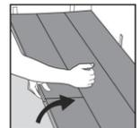
Slide the ends in opposite directions to disengage. Do not pull upwards to disengage the short ends so as not to break them
